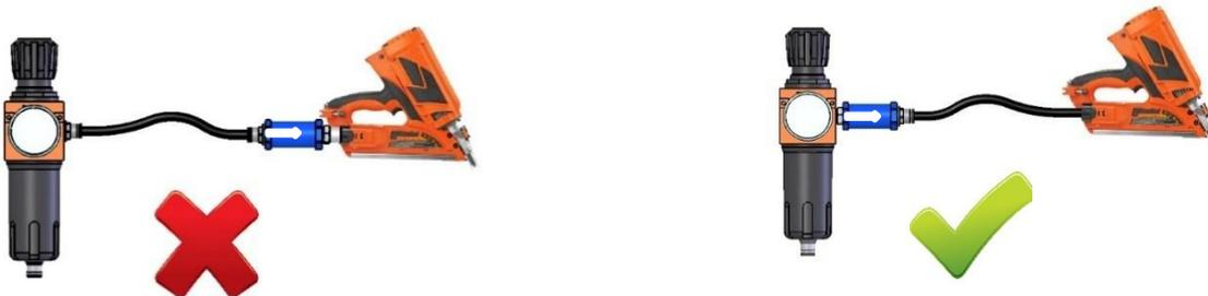
The HoseGuard **must** be mounted at the end of a rigid feeding line
